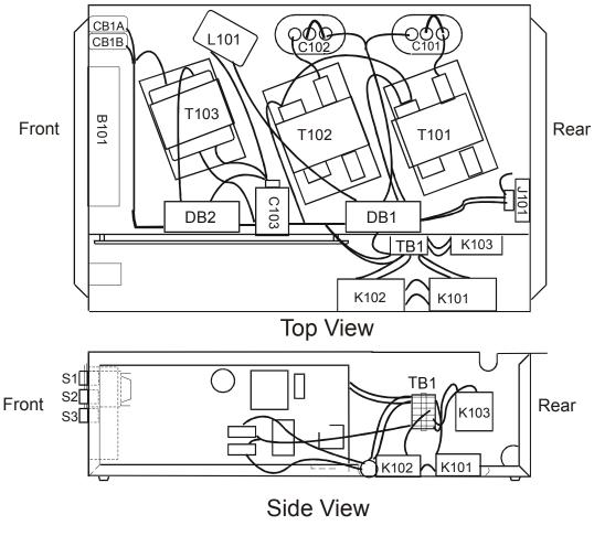
Figure 45. P300M/P300MQ HV Wiring
